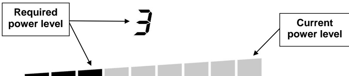
The segments from the power display are turning off one by one until the required power level is reached.
